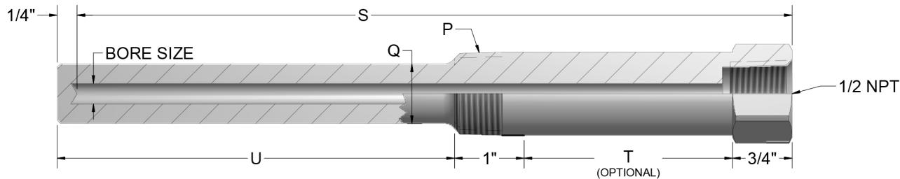
Wells are made from round bar with milled wrench hex. 1 1/4" NPT and 1 1/2" NPT wells are supplied as round bar with milled wrench flats.
